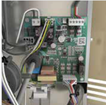
DSI Control Board designed for easy servicing
