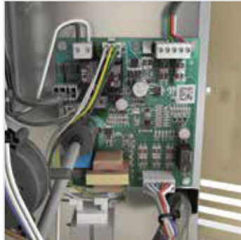
DSI Control Board designed for easy servicing
